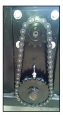
New larger #80 drive sprockets & chain increased from #60 for added strength & longevity.
