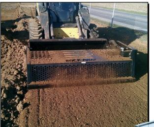
Affordable, low maintenance, quality landscaping tool for virtually any skid-steer loader. ROCKAWAY picks rocks in reverse, but can also push small amounts of dirt moving forward. Low profile makes visibility excellent!
