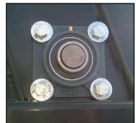
duty, 1 3/8" bearings. Rotor has been redesigned with a bolted hub for easy service.
